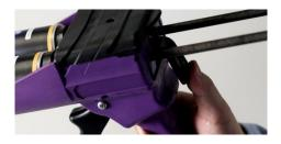
5. Always press the spring plate when you want to stop the grout flowing out.
