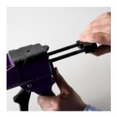
2. Prepare the caulking gun correctly as this picture shows before putting the cartridge in. One thumb presses the spring plate. Meanwhile the other hand pulls backwards the propelling rod. Don't press the trigger at this time.
