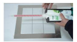
3. Install the cartridge into the caulking gun. Make sure to lock the slot of the cartridge onto the rail of the gun, as this picture shows. It's important.
