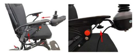
② Ensure that the Controller plug is properly connected to the battery.
