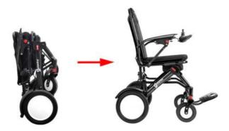
② Press the fold button between the seat and the battery to make sure it is locked. Pull hard to ensure the lock clicks in place.
