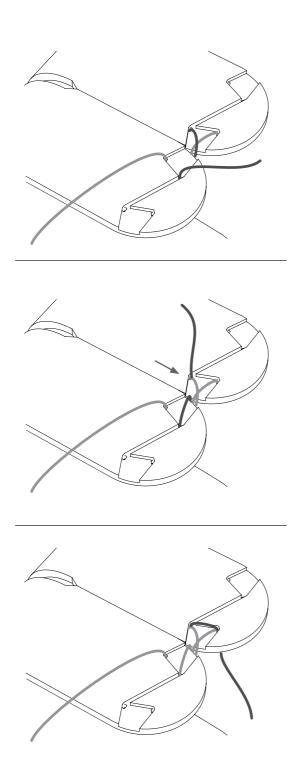
Thread the cord downwards between the parts and pull it upwards through the front hole of part 1.
