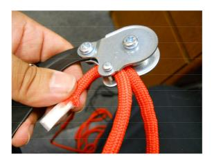
STEP 4: Insert rope on wood handle, make a knot, and cut excess as needed.
