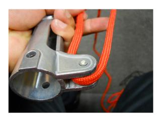
STEP 3: Insert rope between rivet and rope and pull enough rope to cramp tight with baker clip. (See "Tying a Rope Knot" video for reference.)
