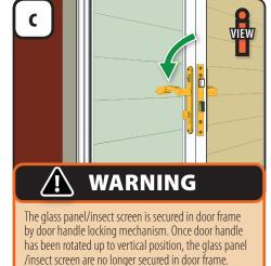
door frame after releasing locking mechanism. Failure to do so could result in injury and/or product damage.
