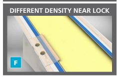
**F.** If you cut near the lock, you will be cutting through material of a different density. You will feel slightly more resistance in this area.
