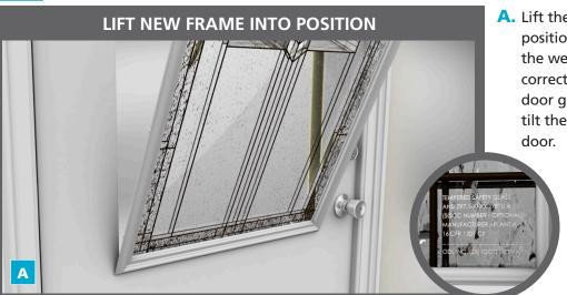
A. Lift the new frame with glass into position from the outside. To ensure that the weight of the glass is distributed correctly, place the bottom edge of the door glass snugly against the door. Then tilt the top into position against the door.
