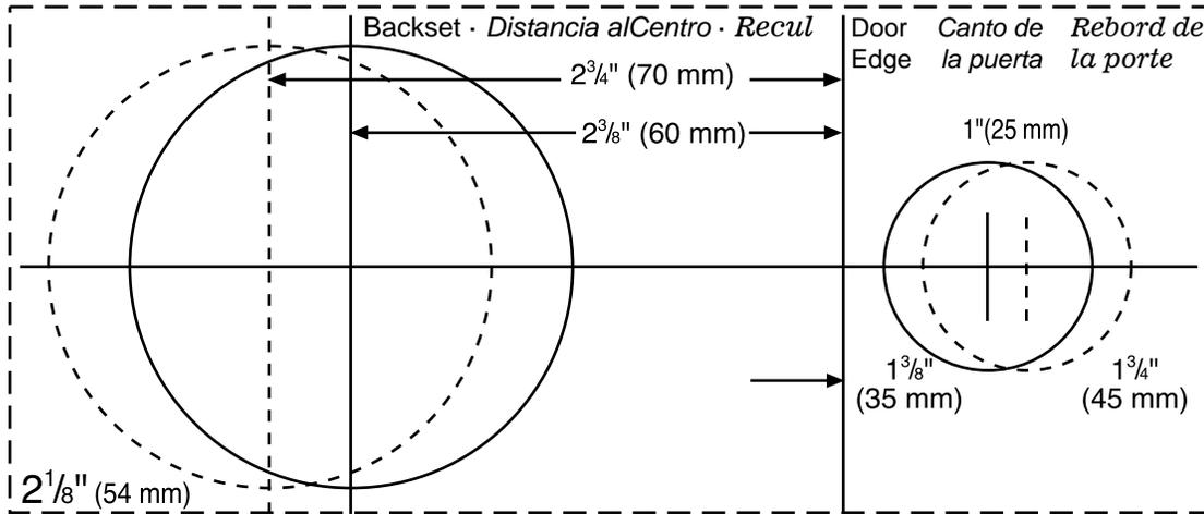
"Backset" is the distance from the door edge to the center of the mounting hole for the door knob or lever.
