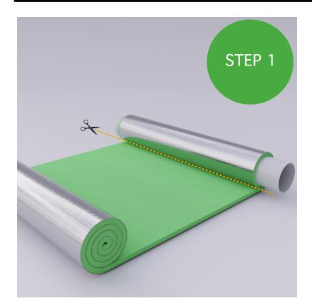
Measure and Cut NuWrap XtraFlex to match the diameter of the pipe, with a ~40mm overlap, so for a 110mm outside diameter pipe cut your width to ~520mm
