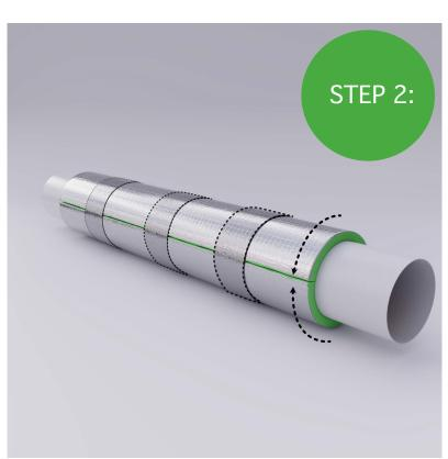
Wrap the NuWrap XtraFlex around pipe. Keep the outside surface clean and dust free. Apply Thermotec Reinforced 72mm wide self adhesive foil reinforced tape around the circumference and joins. On horizontal pipes rotate the join to face downwards.
