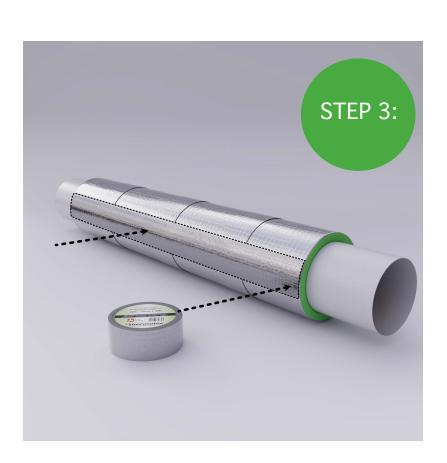
Apply the Thermotec Reinforced 72mm wide self adhesive foil tape lengthwise along the join. For the best acoustic performance, make sure there are no gaps between any of the joins.
