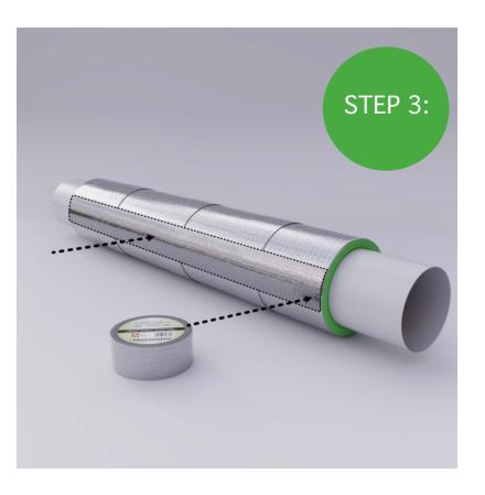
Apply the Thermotec Reinforced 72mm wide self adhesive foil tape lengthwise along the join. For the best acoustic performance, make sure there are no gaps between any of the joins.
