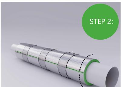
Wrap the NuWrap 5<sup>(TM)</sup> around pipe. Keep the outside surface clean and dust free. Apply Thermotec Reinforced 72mm wide self adhesive foil reinforced tape around the circumference and joins. On horizontal pipes rotate the join to face downwards.
