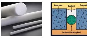
Thermotec Closed Cell Backing Rod is manufactured from closed cell low density polyethylene foam. The product is manufactured in a range of sizes and has excellent compression and recovery properties
