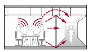
NuWave\* will need to be installed so that all penetrations, material overlaps, interface with the soffit and the back of the ceiling are sufficiently detailed with respect to acoustics. Furthermore, the extent of the plenum, including the likely amount of return, will/may need consideration to facilitate the final acoustic outcomes.
