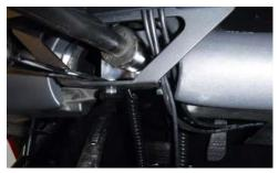
• Using a 1/2" wrench, tighten the mounting bracket on to the steering column bracket bolts with the provided non-locking nuts.
