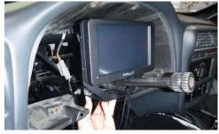
Position the steering column brackets, mounting bolts, and the dash/mounting bracket assembly in the required location.
