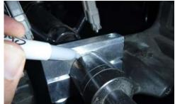
• Remove the Holley dash and mounting bracket, then mark your desired steering column bracket location on the steering column.
