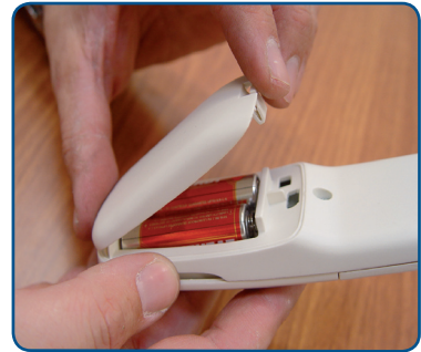
Fig. 4.1: Changing the batteries of the call and send stations.
