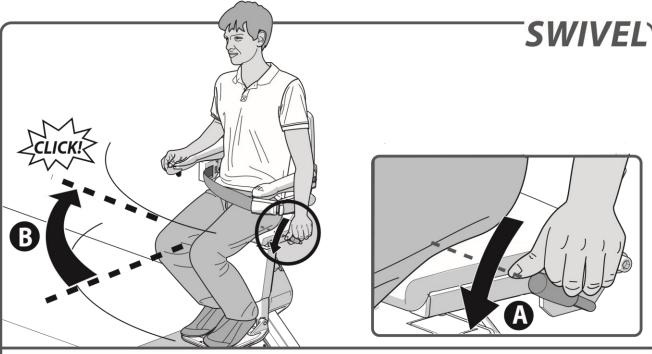
The lift stops automatically at the end of the rail. You should now swivel the seat manually, making it easier to get on and off. To do this, push down the lever{A}. Swivel the seat until you hear a 'click'. The seat is now in the correct position{B}.
