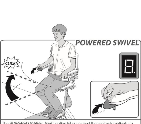
The POWERED SWIVEL SEAT option let you swivel the seat automatically to face the direction you are going to walk. To do this, push and hold the joystick in the direction of travel.
