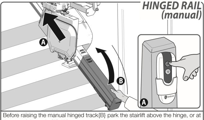
the top of the stairs{A}. When your stairlift is not in use it should always be positioned away from the hinged section with the hinge in the raised position.
