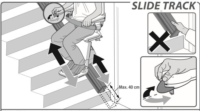
If the lift has a sliding track, both the chair and slide track will move at the same time. Once the slide track has reached the end of its travel the lift will continue its travel. Keep the toggle pressed in the same direction.
