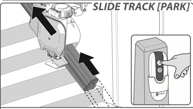
When the lift is not in use it should be moved away from the bottom of the stairs so that it does not cause an obstruction. To park the lift, press and hold the UP button on the handset.
