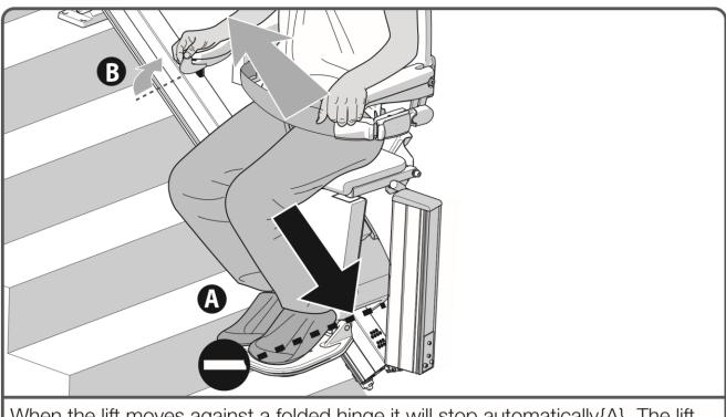
When the lift moves against a folded hinge it will stop automatically{A}. The lift can still ride in the upwards direction{B}.
