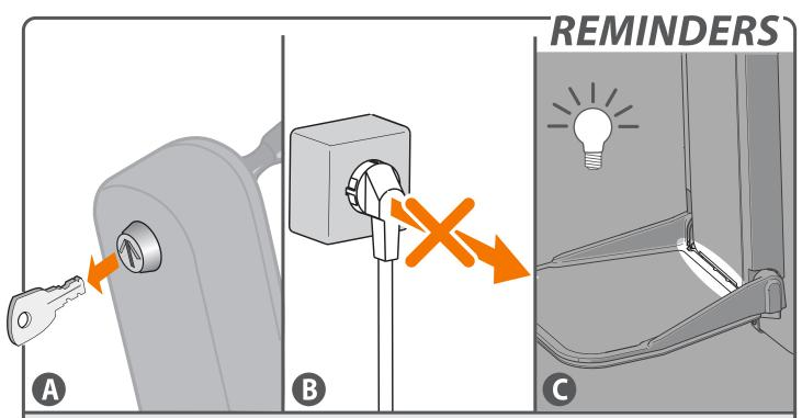
[A]Remove the key from the switch whenever you leave the lift.
