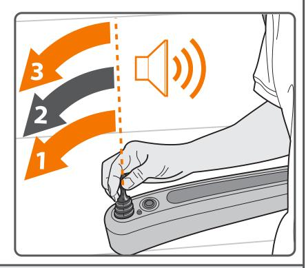
Stairlift with powered swivel can swivel automatic on a preferent intermediate landing after tapping. Before the start of the lift, the joystick (not the remote control) is operated in the direction of travel (Tap). The number of operations (taps) indicates the desired floor. Tapping must be done rather quickly. After each tap you hear a beeping sound. LAST press (when holding the joystick to start driving) is NOT counted as a tap!!
