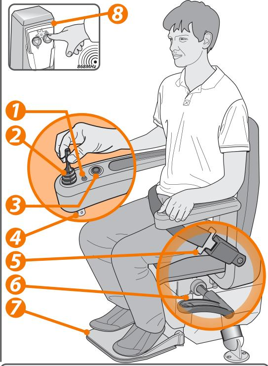
The illustration opposite shows the features used to operate the Classic seat. The Classic can be upgraded with the automatic swivel seat, powered footrest, hinged rail, Turn & Go, Voice Connect and Active Seat options to create even more seat comfort and user-friendliness.
