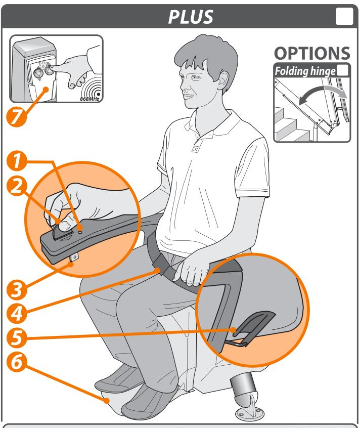
The illustration opposite shows the features used to operate the Plus seat. The Plus seat can be upgraded with a hinged rail, making it more user-friendly.
