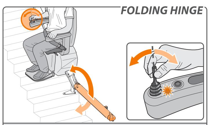
With the FOLDING HINGE option, the seat stops just above the hinged rail. Move the joystick up or down to fold or unfold the rail.
