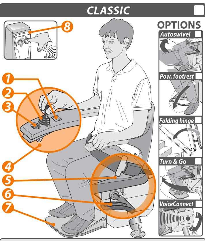
The illustration opposite shows the features used to operate the Classic seat. The Classic can be upgraded with the automatic swivel seat, powered footrest, hinged rail, Voice Connect and Turn & Go options to create even more seat comfort and user-friendliness. [1]LED
