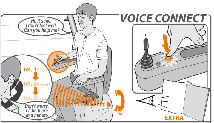
The VOICE CONNECT option lets you call one of the three telephone numbers you have chosen, by pressing the red button. Check once a month that the Voice Connect function is working correctly. For more details, please read the separate Voice Connect documentation.
