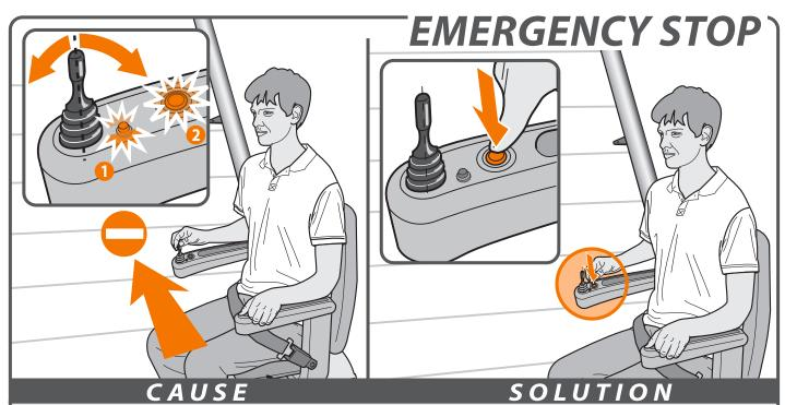
Problem: the lift does not travel in either direction, the LED[1] flashes when the
