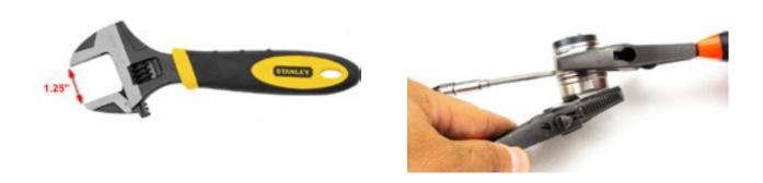
The wrenches should provide enough force to unscrew both parts from eachother.
