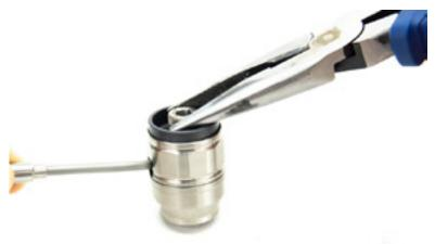
Using some rags, try to unscrew the diffuser from the head by hand. If this attempt fails, go to the next step.
