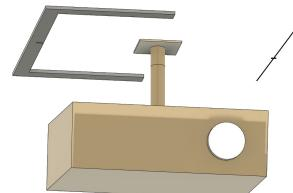
Strike line on ceiling along inside edge of guide, marking center point
