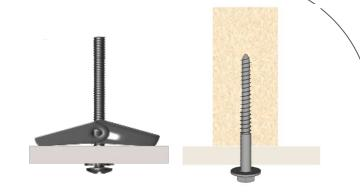
Where no joist, drill 5/8" hole for toggle bolts.
