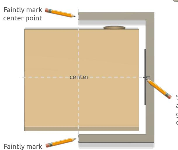
Strike line on ceiling along inside edge of guide, marking center point
