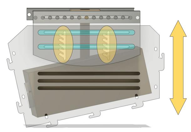
The two vertical notched slots on the projector shield allow for different drop heights.
