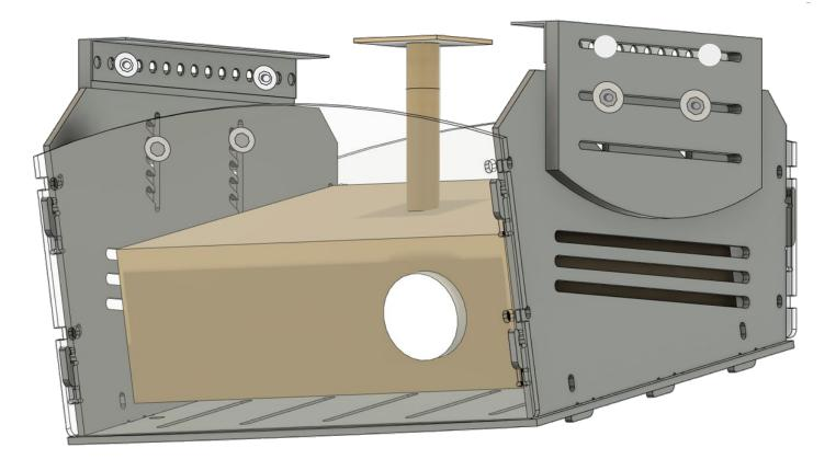
The horizontal slots on the drop brackets allow the projector shield to slide forward or backward for centering the projector.
