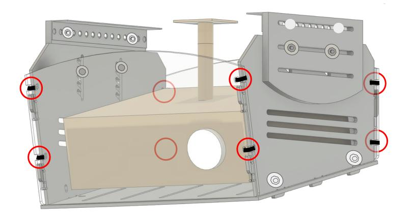
It is important to install these safety straps to keep these panels secure if shield is impacted by balls or clubs.
