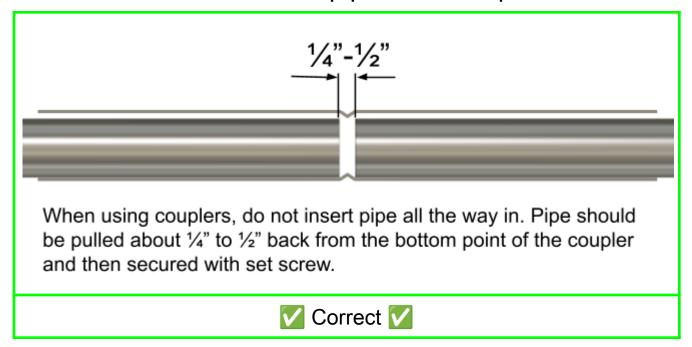
Do not insert pipes all the way inside couplers. Pipes should be secured into couplers about  $\frac{1}{4}$ "- $\frac{1}{2}$ " from bottoming out inside of couplers.
