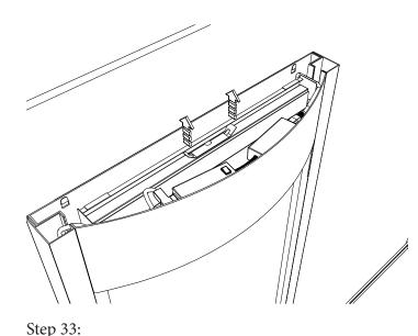
Reinstall the Baffle into the Water Distribution Unit
