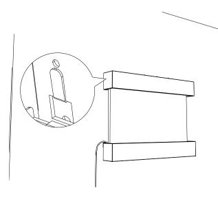
The Water Surfaces are designed to allow for some adjustments by hand, if needed, to help with the water flow. By placing your hand behind the Water Surface, you are able to wiggle the stone slightly if needed to allow for proper water flow.
