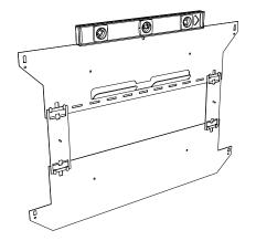
Step 67 Use a Carpenter's Level to ensure that the Bracket is level.
