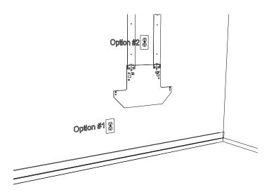
There are two options where the Electrical Outlet can be located, either below the Tray or behind the Water Feature. If you decide to wire an outlet behind the Water Feature to allow for a concealed Power Cord, this is the area you want the outlet to be. We also recommend wiring the outlet to a wall switch for ease of turning the Water Feature on and off.
