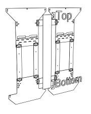
Some Multi-Panel Features have a decorative Cover Panel. The top of the Cover Panel is the side with the least amount of space between the notches and the end.
