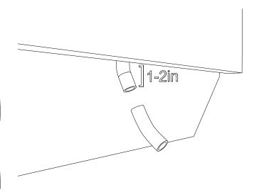
Step 34 The Hose should be cut to allow approximately 1 to 2 inches below the bottom of the Slab.
