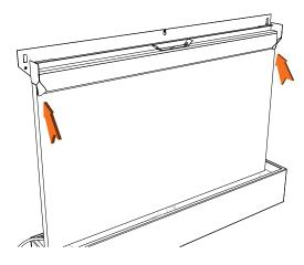
The outer edge adjusting tabs are used to control water flow at the edges of the Stone. If there is a large amount of water flow at one or both edges you may experience a small amount of water dripping off these tabs. If this occurs, simply bend the tabs by hand in to redirect the water onto the Stone. The tabs should be bent in to touch the front of the Water Distribution Unit.
