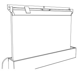
Clean the front surface and top lip of the Water Distribution Unit with the supplied Scotch Brite Pad. Rub the Pad back and forth on the entire surface until it is noticeably cleaner and shinier.
