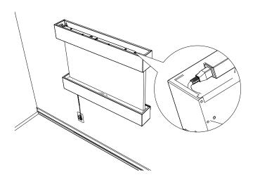
Step 103 Plug in the Pump Power Cord to the outlet on the Hood.
