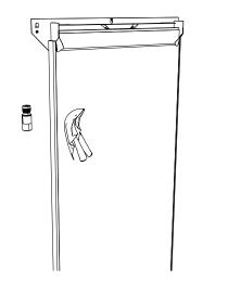
If you have a mirror or Glass Surface, add a small amount of the Mirror Prep liquid to a wet rag. Apply the Mirror Prep over the entire surface and let dry for a few minutes. Once dry, remove any excess with a clean wet rag.
