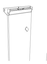
Once the Water Distribution Unit is set, turn off the Water Feature and lightly go over the Unit and Stone with the Scotch Brite Pad while it is still wet. This will help the water completely cover the Stone.
