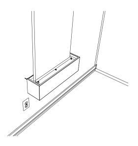
Before installing the Pebble Beach Shelf be sure to bend it a little to allow it to fit into the Tray. Slide the Shelf into the Tray until the upward pointing front lip is secured under the front edge of the Tray. Note: The Pebble Beach Shelf is made of a spring-style plastic. The tension from the plastic is used to hold the Shelf in place. If the Shelf is out of the Tray for too long, it can begin to straighten and may need to be bent back into shape with your hands.
