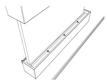
Ensure there is a 1/8in gap between the Stone and the Pebble Shelf back lip. Adjust the back lip of the Shelf by loosening the Screws. This gap will make sure the water will flow without splashing.
