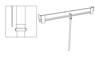
Fasten the Hose to the copper piping on the Water Distribution Unit. Ensure the end of the Hose is pushed past the lip where the copper piping widens. Then use the supplied Hose Clamp or Zip Tie to strengthen and tighten the fitting to ensure that no water can escape.
