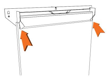
Reinstall the Baffle into the Water Distribution Unit and bend the upper copper tabs back into place. Do not force the tabs up. Bend them up until the Baffle will not come out of the Unit, but still has a little room to move.
