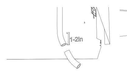
The Hose should be cut to allow approximately 1 to 2 inches below the bottom of the Slab.
