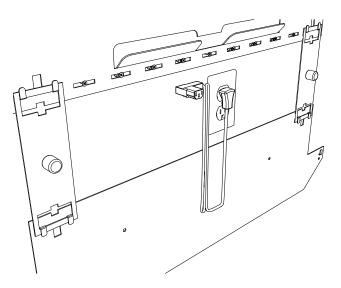
If using an outlet behind the Water Feature, plug in the white Power Cord before hanging the Water Surface.
