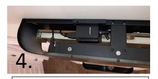
4. Tuck the cords behind the water distribution unit and adjust the location of the receiver to allow for operation.
