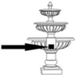
FT-239G (2 lbs) pump house doors
