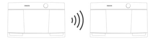
Once the two speakers are paired, press the LINK button to cycle through the channel modes. Choose from (L)(R), (L), or (R). Control the audio through the master speaker (the one without the SATELLITE icon illuminated) by using the onboard controls or the music source.
