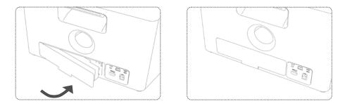
There is a small latch on the bottom of the unit that keeps the battery in place. When installing the battery, insert the tabs on the left first, and push the battery in until the latch clicks. To remove the battery, pull the catch on the latch outward.
