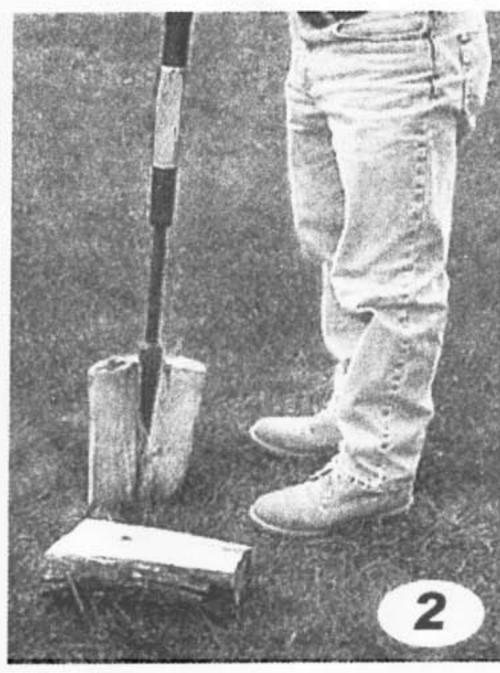
Raise the sliding hammer handle of the splitter with both hands. Keep feet safely away from the base of the log.
