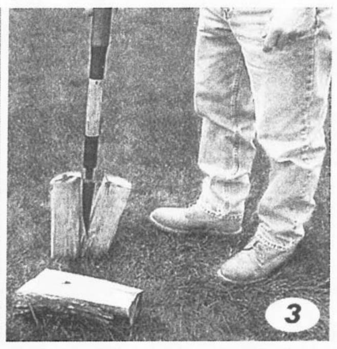
Push the sliding hammer handle down with quick force to drive the wedge into the log. (TIP: Start wedge into log by a tap first before using full force.)
