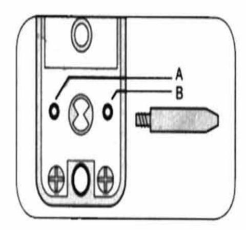
(4) Position Door Template and Drill Mounting Post Hole.
