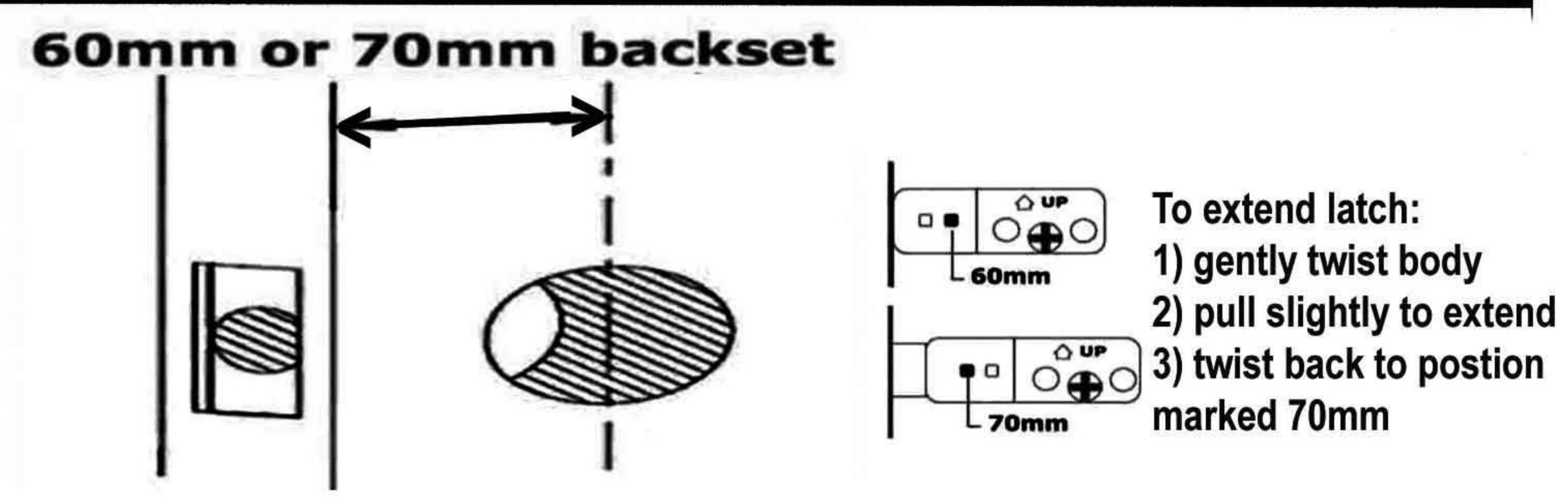
Installation Note (D): Adjust Latch for Backset 60mm or 70mm
