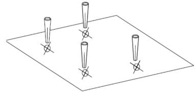
7. Align the holes of the stand with the holes on the floor and use the M8x75mm hexagon tapping bolts to tighten.
