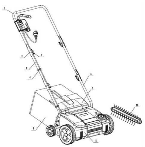
1. Upper Push Rod2. Bolt3. Middle Push Rod4. Cable5. Knob6. Lower Push Rod7. Tailgate8. Motor Housing9. Straw Frame10. Raker Cylinder10. Raker Cylinder
