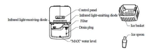
Note: If the 'Ice Full' sensor is lit up, but the machine is not full, please clean the sensors.
