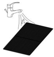
Pic2. Rinse the air filter under running water.
