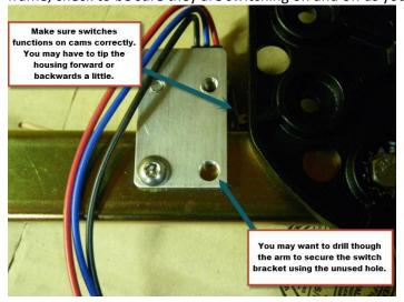
Now reassemble your shifter and connect the wires as marked, make sure your 12V+ supply is on a key on fused source. The two connected black wires are for your 12V+ supply.
