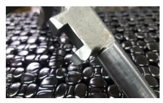
You will want either silicone or use the factory transfer case lever housing gaskets.
