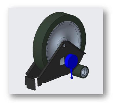
CRITICALLY IMPORTANT: BELT GRINDER MUST BE RUN IN REVERSE (BELT TRAVELING UP THE FRONT OF THE CONTACT WHEEL) IN ORDER TO PREVENT SERIOUS INJURY TO THE OPERATOR OR DAMAGE TO THE EQUIPMENT.
