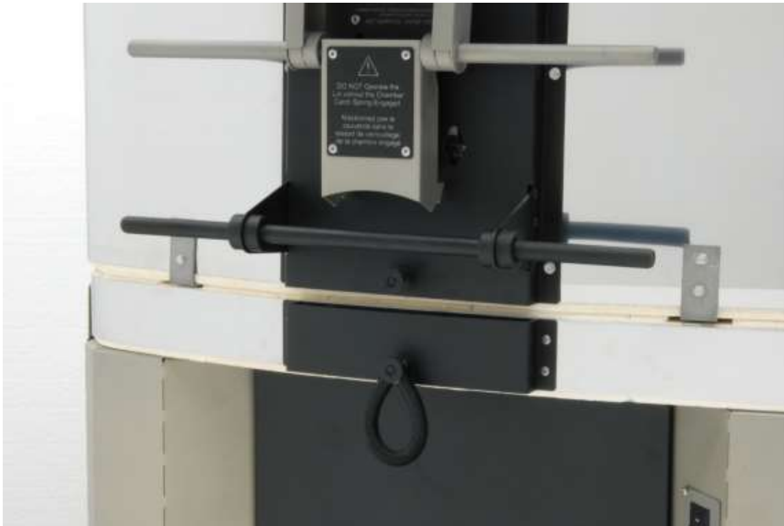
Figure 2 - Chamber Safety Catch Unsecured
