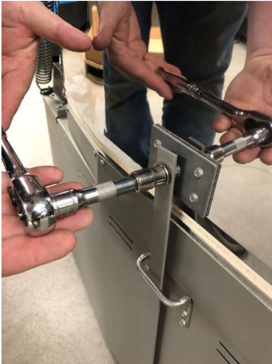
Figure 78 - Chamber Safety Bar Installation
