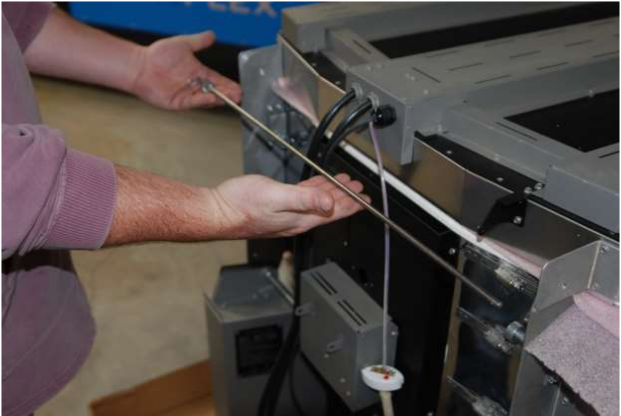
Figure 19 - Hinge Rod Removed
