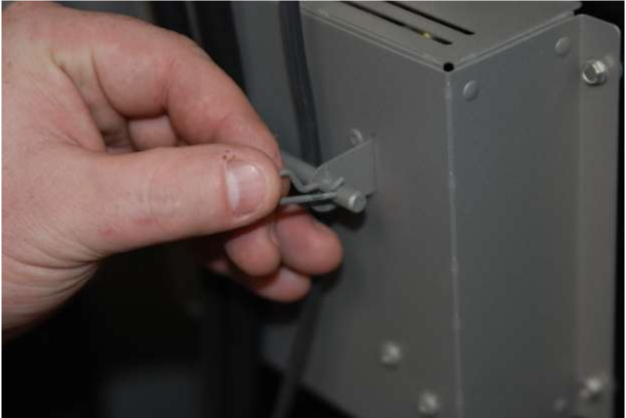
Figure 58 - Cable Management Rod
