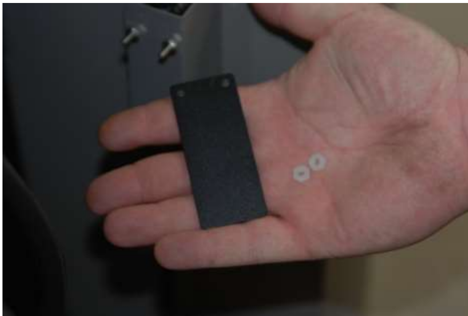
Figure 90 - Power Interrupt Switch Gauge
