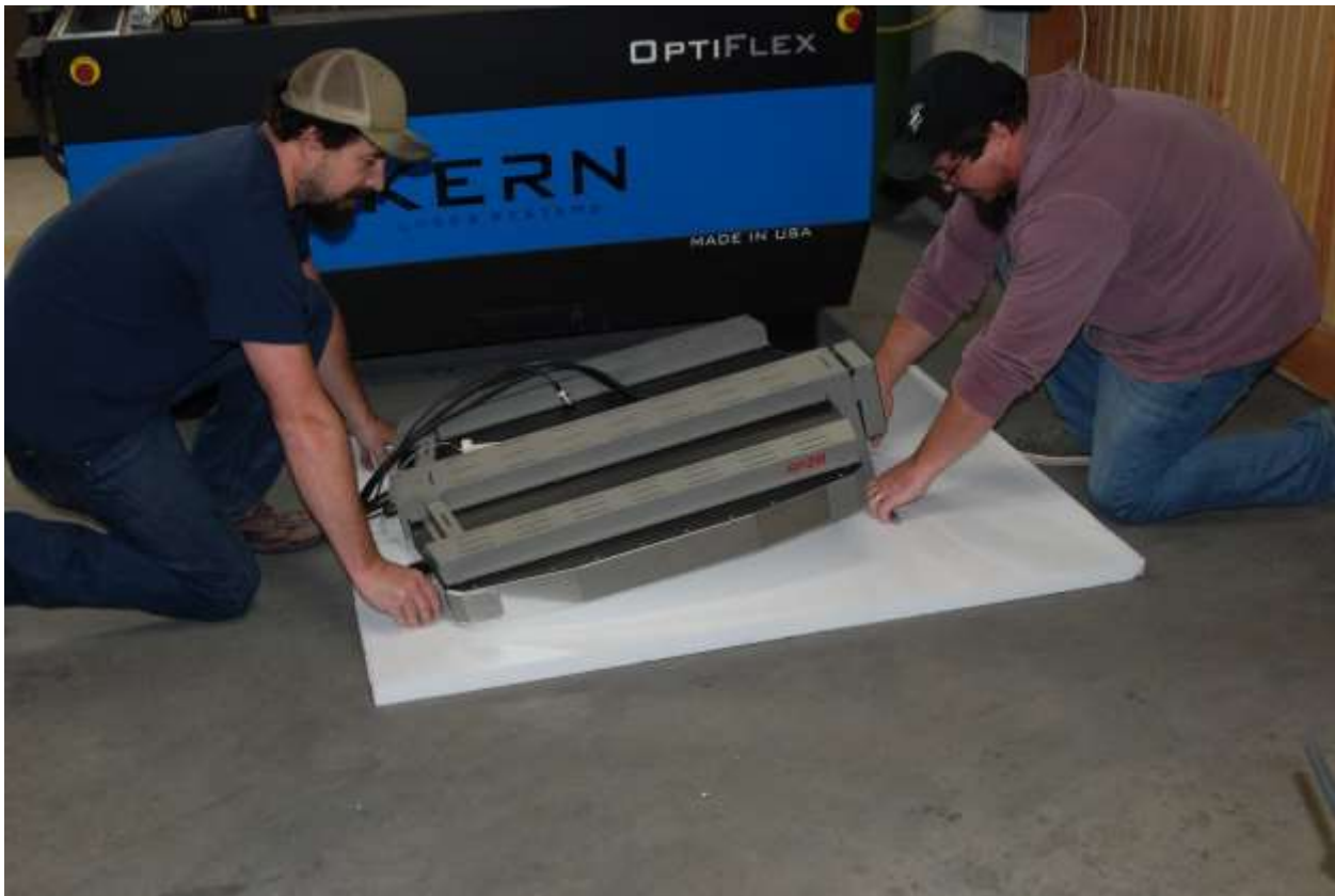
Figure 24 - Placing Removed Lid Down
