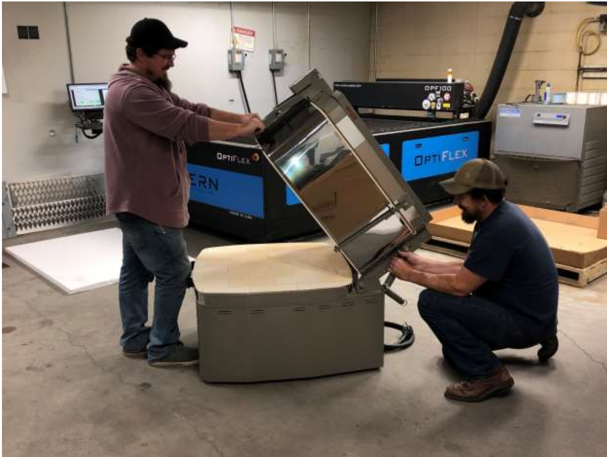
Figure 82 - Lift Assist Spring Installation SP28 and SP41
