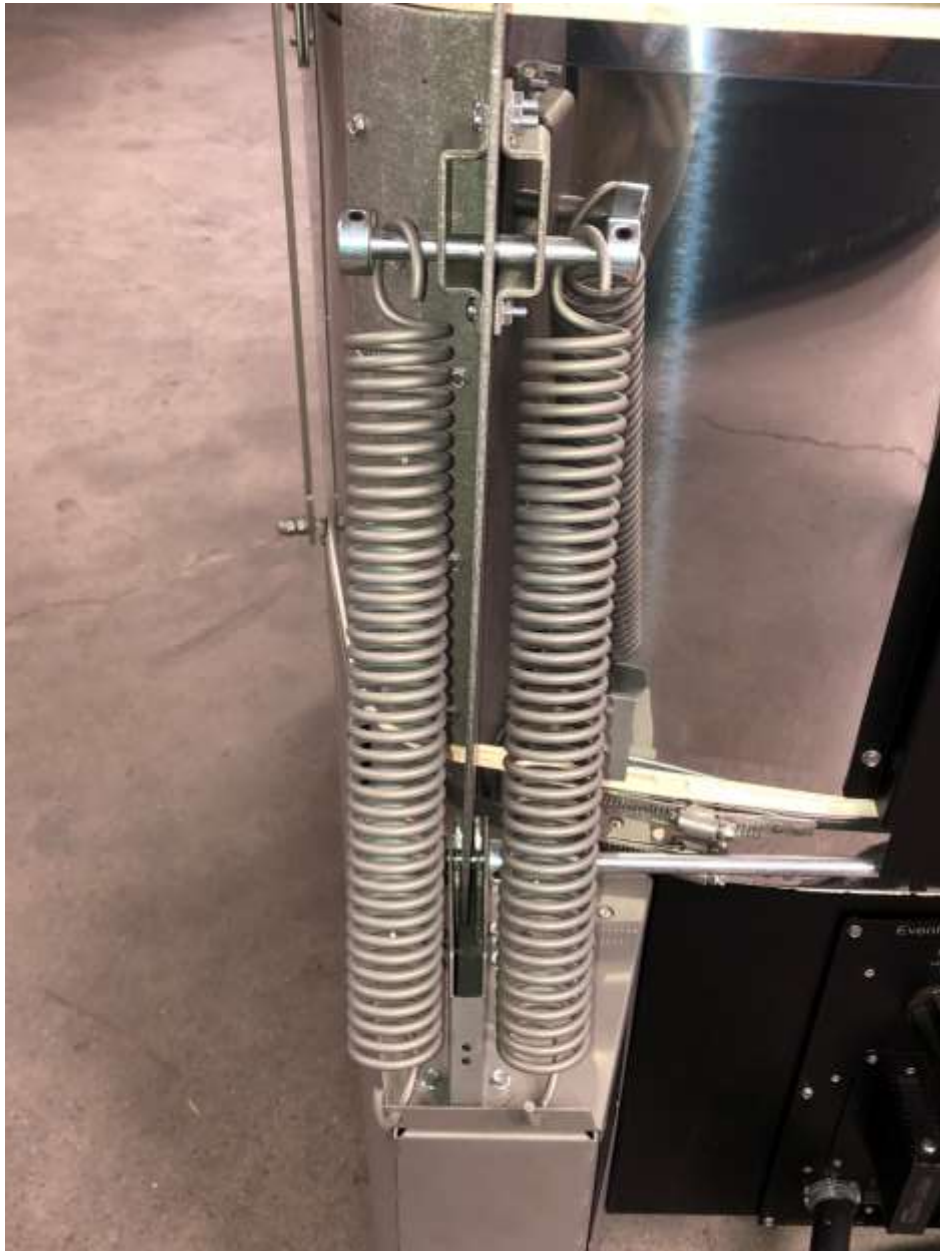
Figure 84 - Lift Assist Spring Installation SP28 and SP41
