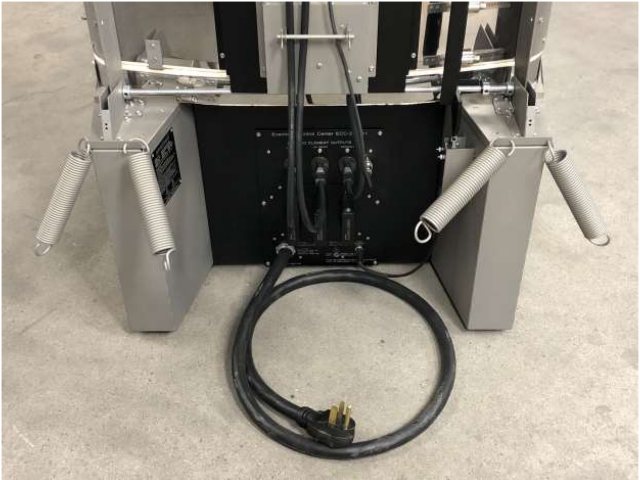
Figure 81 - Lift Assist Spring Installation SP 28 and SP41
