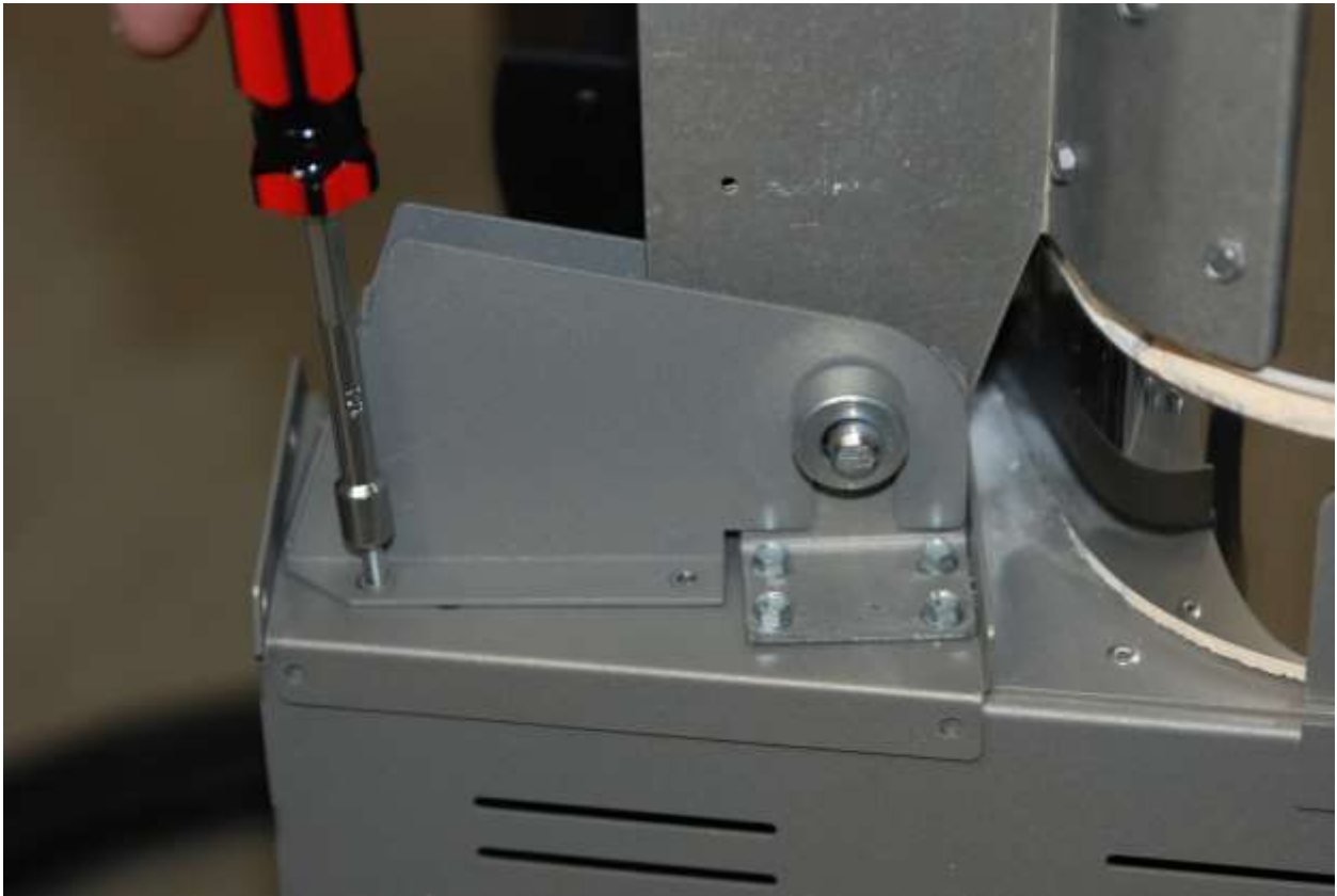
Figure 47 – Re-install Counter Yokes
