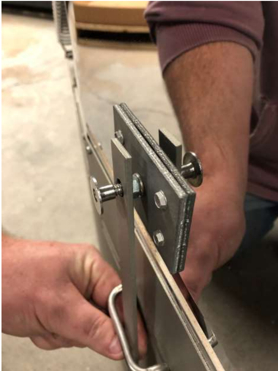
Figure 76 - Chamber Safety Bar Installation
