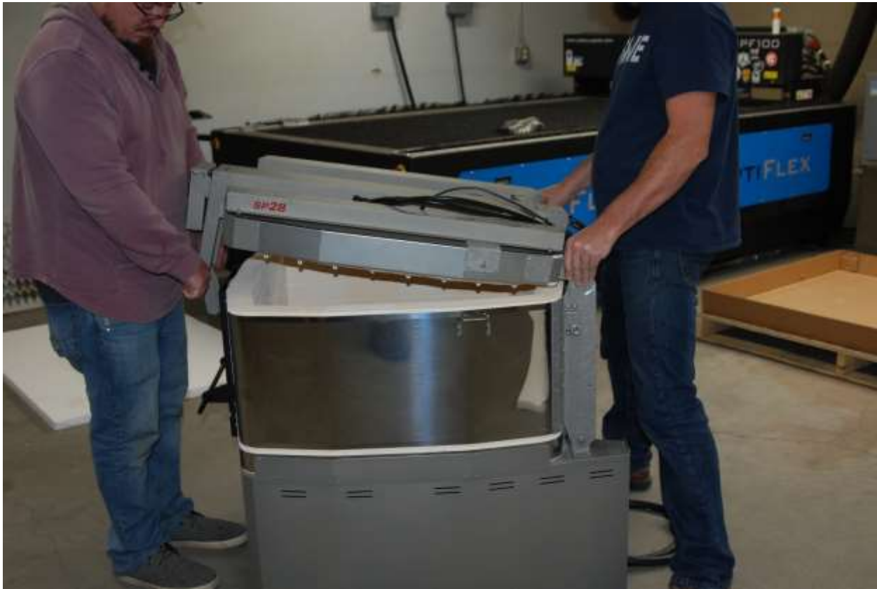
Figure 46 - Placing the Lid on the Chamber
