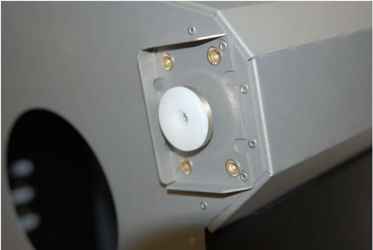
Figure 39 - Leveling Feet Attached
