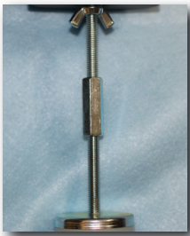
Completed Fixed Position Pedestal
