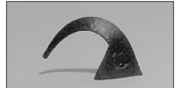
A self-supporting cone fired to maturity. Do not be concerned if the tip is slightly higher or lower than shown.
