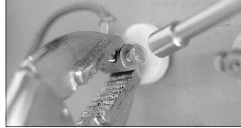
Hold the element connector with locking pliers when removing and installing the connector.
