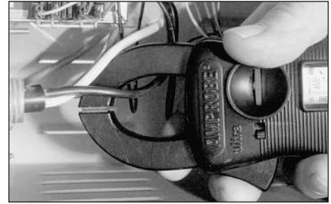
The ammeter attaches to only one cord set hot wire. Be sure breaker is shut off before you remove the kiln's switch box. DO NOT TOUCH WIRES after you turn the breaker on.
