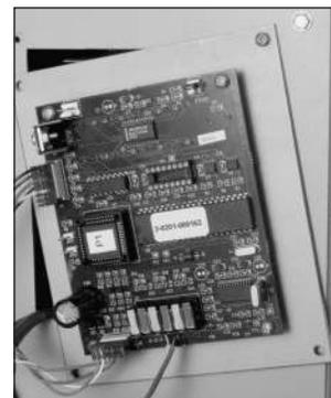
Disconnect power before removing the board from the switch box.
