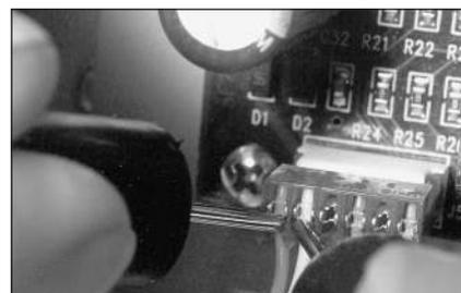
Testing for voltage at the controller's INPUT terminals.
