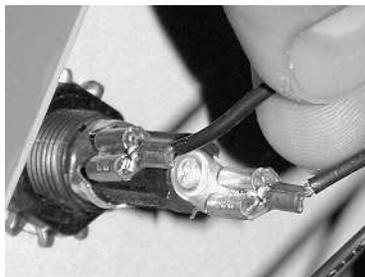
Checking the push-on connectors for tightness on the ½ amp fuse holder.
