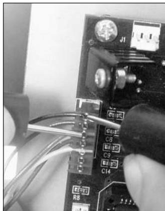
Testing for voltage at the red and black output wires on the back of the Sentry.
