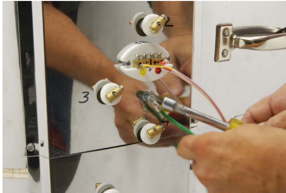
Step 4 – Disconnect the green ground wire connecting the control panel to the kiln, at the kiln. Use an 11/32" tool to remove the fastener.
