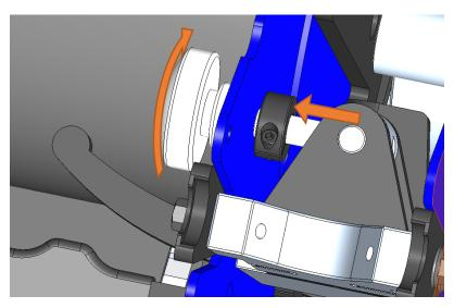
Make sure the small wheel holder does not display any free movement when pushed by hand. If there is free play and the tracking knob is already tensioned as described in the previous step, make sure all of the fasteners indicated below are tight in the small wheel holder (mating parts hidden for visibility)
