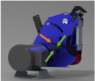
c. Spin the belt by hand for 2 to 4 full revolutions in the forward direction while roughly adjusting the tracking knob as indicated below to ensure the belt will not collide with the blue frame when the motor is started
