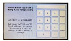
Enter ramp rate in degrees per hour. For maximum rate enter 9999
