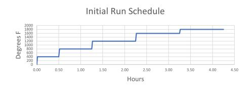
400°F for 30 minutes 800°F for 45 minutes 1200°F for 60 minutes 1600°F for 60 minutes 1800°F for 60 minutes
