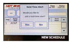
Adding a hold time alert will sound an alarm when the segment hold time has completed.
