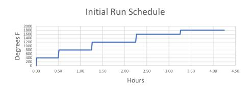
400°F for 30 minutes 800°F for 45 minutes 1200°F for 60 minutes 1600°F for 60 minutes 1800°F for 60 minutes
