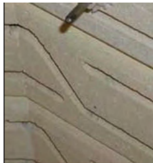
Thermocouple will show through brick wall at a maximum of 1". Pack kiln sitter hole with ceramic fiber to seal it.
