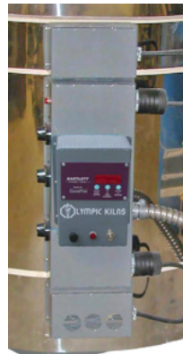
Install Electro Sitter in the same location as the former kiln sitter plate.
