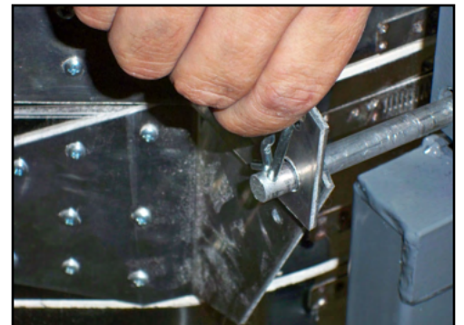
Position armlifter holes to match back of vertical back support holes and holes of lid. Insert stiffening strut through holes and lock in place with cotter pin.
