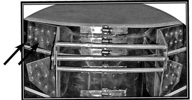
Repositioning Lid when Thermal Expansion Occurs
