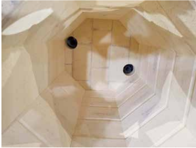
Inside a Torchbearer 1827G with bottom lined up correctly over gas burners
