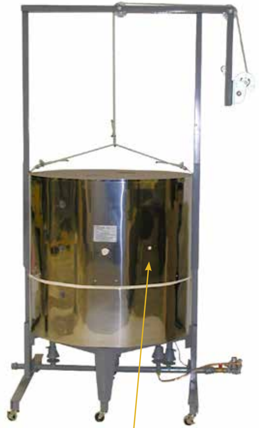
Exposed area in stainless steel jacket
