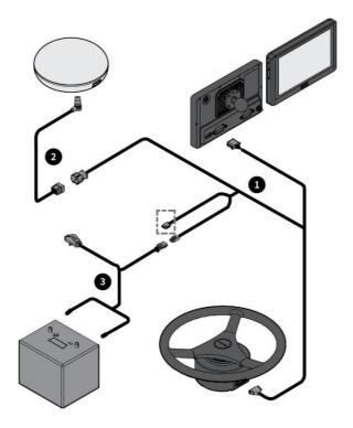
The diagram above is showed that the connection of main components of Sveaverken F100 Auto Steer System by main wiring harness **1**, GNSS receiver wiring harness **2**, main power cable **3**.
