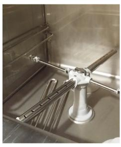
Various machine models require additional cleaning of wash and rinse arms during normal operation. This is to ensure that correct water flow is reaching the wash items. Contact Warewashing Solutions on 1300 217 411 or go to www.warewashingsolutions.com.au for standard operating instructions
