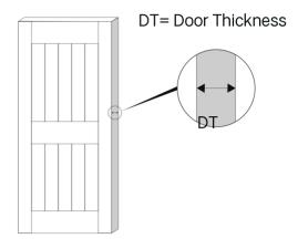
Check your door thickness. If it is 1-5/8" or less you can mount the bracket against the wall while mounting on the ceiling studs. If it is more than 1-5/8" thick, the bracket has to be mounted further from the wall on the ceiling.
