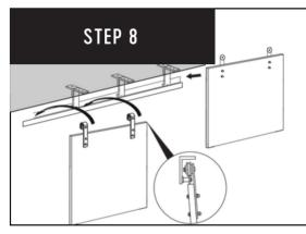
To mount your doors on to the track, you will have to lift your door at a slight angle and rest both wheel grooves onto the top of the track carefully. For the track nearest to the wall you will have to slide it from one side but make sure to take out the door stopper for the side you are about to slide it in to.
