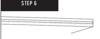
Route a slot that is 1/4" wide and 1-3/16" deep at the bottom of the door for all three doors. If you do not want to open a slot underneath your doors, we provided a 2-in-1 floor guide which will show 2 mounting ways on step 11. If you would like to purchase special floor guides not provided you can look up "floor guides" in the search bar of our website to see all the types of floor guides we sell.
