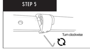
Install the door stoppers on each end of the track like the diagram with the hex wrench. This door stopper is adjustable. You can change up the position however you like by just sliding it on the track and tightening it where you need it to be. It slides over all lag bolt head making it easy to install.
