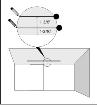
Make sure you have ceiling studs for this setup! Use a leveler to make sure your ceiling is leveled. Draw 2 lines on the ceiling parallel to the wall. Line 1 is 1-3/16" away from the wall and Line 2 is 13/8" away from line 1.
