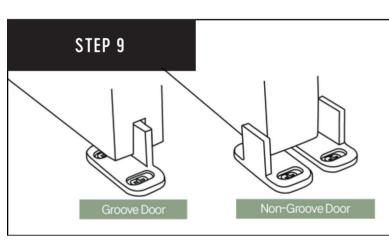
For the floor guides of we recommend to install the regular floor guide in your own location preference depending on how you want your door to slide. Here below is a diagram of the 2 ways you can use the given floor guide. If you are looking for different floor guides please check out our website. Type in "Floor Guide" in the search bar of our website and you will be able to find a few types.
