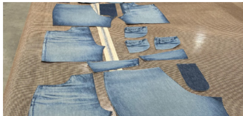
Laser-cut and -faded pieces for Everlane shorts, ready to be sewn together. Photo: Dhani Mau/Fashionista
