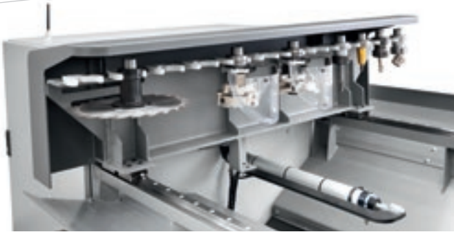
Rack tool magazine with 12 places.
