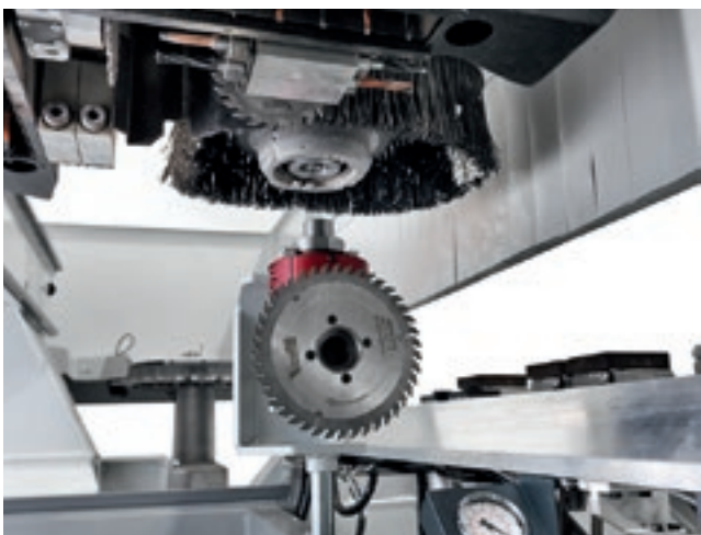
The Pick Up station supports automatic tool-holder rack tooling.
