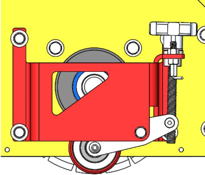
3. Raise the machine by using the T-handle until the drum is off of the ground.
