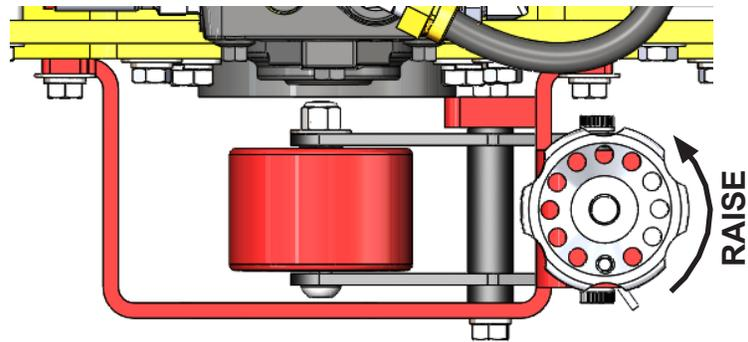
3. Make the next pass. This pass should have the same cut depth as the previous pass. Adjust the height adjustment wheels as necessary to achieve this result.
